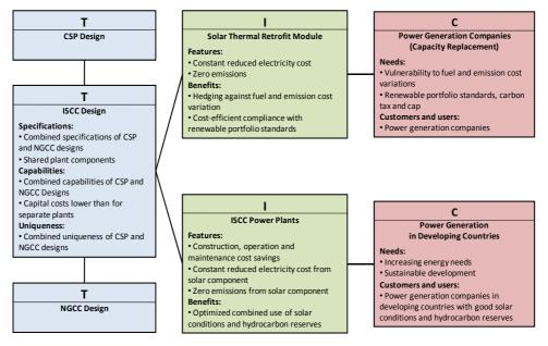
The combination of the CSP and NGCC designs results in a new integrated solar combined cycle (ISCC) design, with the technical advantages of the original designs and
